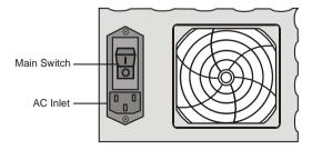
2. Insert the power cable into the power source socket.
